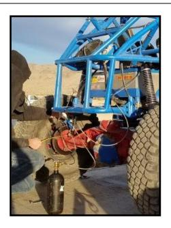
3.1.4 Once pressurized and level, 160cc oil (included in Level-It) from each Level-It cylinder will transfer automatically to each shocks/struts while driving and cycling of the suspension.
