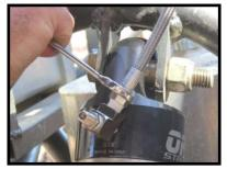
2.5 For integral or remote reservoir *(not piggyback)* struts, order PA-235-D adapter kit to provide needed clearance between T-fitting and compression damping knob.
