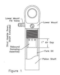
8.2.4 Unscrew and remove lower mount and rebound damping assembly.
